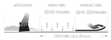
If preferred, the floorcovering or profile can be pre-coated the day before installation. The open time for flooring/ profiles already pre-coated on the previous day into the newly applied film is approximately 90 minutes. The surfaces coated/pre-coated with ARDEX AF 620 must be placed together within the open time of 24 hours.
