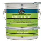
**ARDEX R 3 E** Moisture Tolerant Epoxy Primer is a two component solvent free epoxy resin for use on concrete and cementitious surfaces that have damp surfaces (e.g. from water spillages or rain) prior to installing ARDEX Levelling and Smoothing Compounds.
