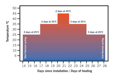
Commissioning of the underfloor heating must not take place until the screed has undergone a minimum of 14 days curing time under normal drying conditions. The water temperature flowing through the pipes must be carefully controlled during a thermal heat cycle, as follows:
